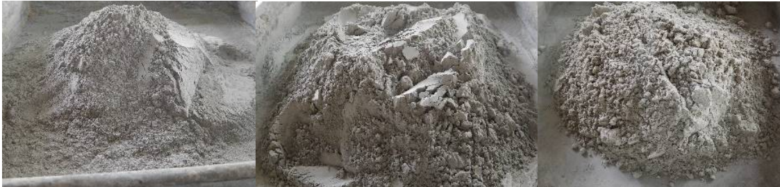
Figure 1: (a) Black Fly Ash, (b) Grey Fly Ash, (c) White Fly Ash
